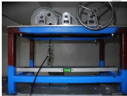
图 5 基于结冰风洞实验段的黏附强度测量装置 Fig. 5 Adhesion strength measurement device based on icing wind tunnel test section
